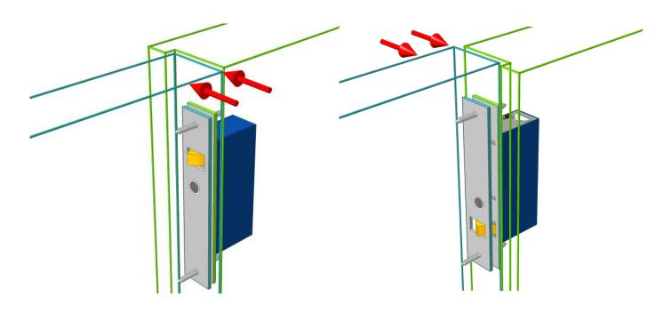
Door closing from the left, the lock is installed with the bolt pin at the top.
